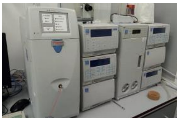
Figure 3. Ion exchange chromatography used for chemical analysis of treated wastewater.
