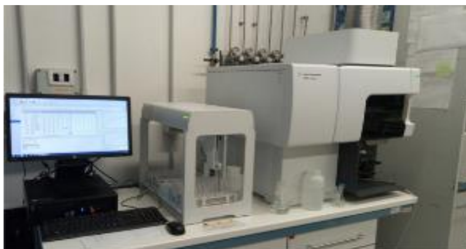
Figure 4. Inductively coupled plasma - optical emission spectrometer (ICP-OES) .
