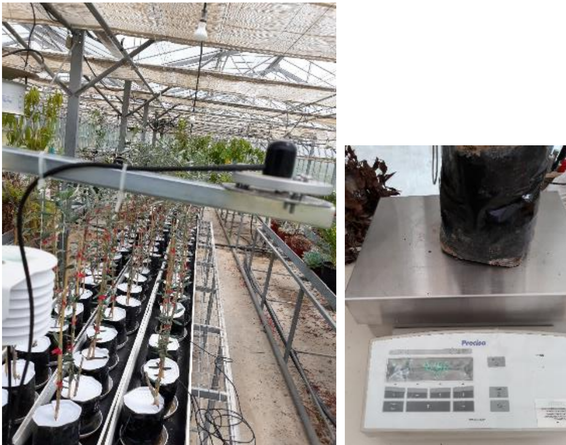
Figure 2 Left: Microclimate monitoring (pyranometer and microclimate sensor). Right: Pot weighing for the determination of daily water needs
