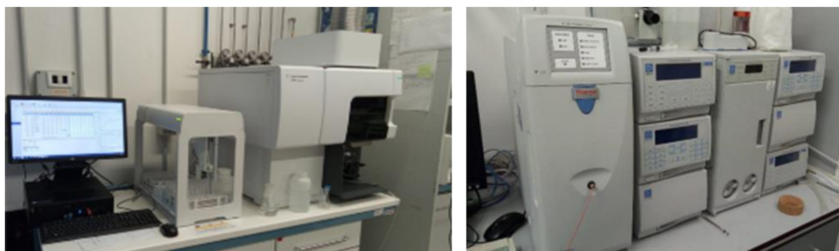
Figure 3. Inductively coupled plasma - optical emission spectrometer (ICP-OES) and ion exchange chromatography used for chemical analysis of treated wastewater.
